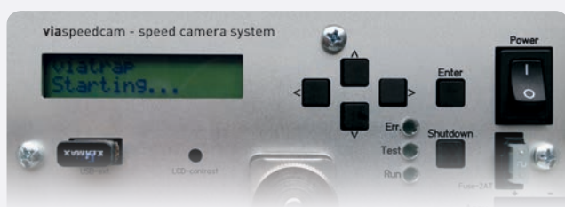
Control panel inside the battery box.
